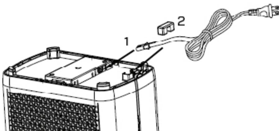
1. Remove the power cord glue from the bottom of the device and insert the end of the power cord into the socket at the bottom of the device (as shown in figure 1).
